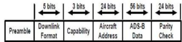
Figure 3. ADS B message format
