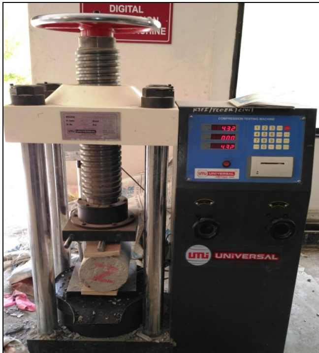
Figure 6. Split tensile strength test setup
