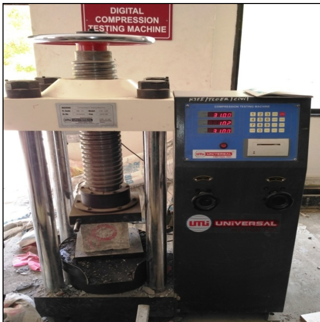
Figure 4. Experimental setup of compression testing machine.
