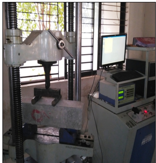
Figure 8. Flexural strength test setup
