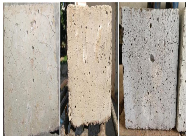
Specimens exposed between 600°C to 800°C
