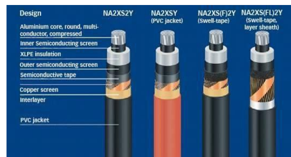
Figure 1. Single core, XLPE insulated medium voltage cables 6kV up to 36kV
