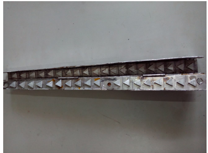
Figure 2. Divergent duct with triangles
