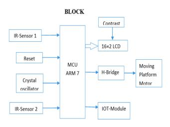
When the train comes near the artificial platform, the proximity sensor senses the train and gives informs to the microcontroller. So that the platform is not connected during the arrival of the train.
