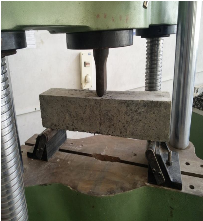
Figure 2. M40 Grade Beam Testing
