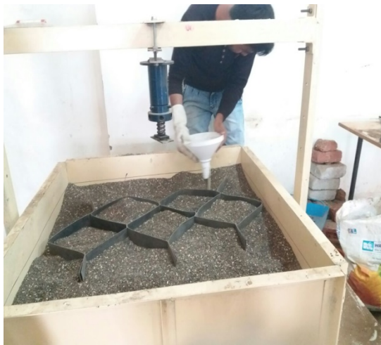
Fig 1. Plate load set up and Expanded Geocell
