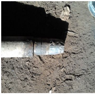
Fig. 4 failed axle of Tractor trolley
