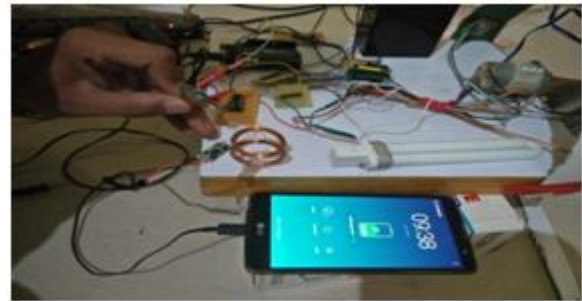
Fig: Wireless power transfer for mobile battery charging
