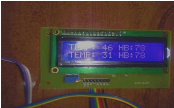
Figure 5. LCD displaying the received Values Heart Rate and Temperature
