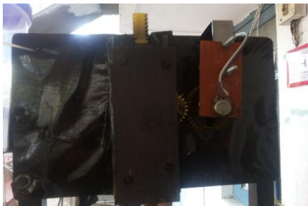
Fig: Feedback control through gear mechanism
