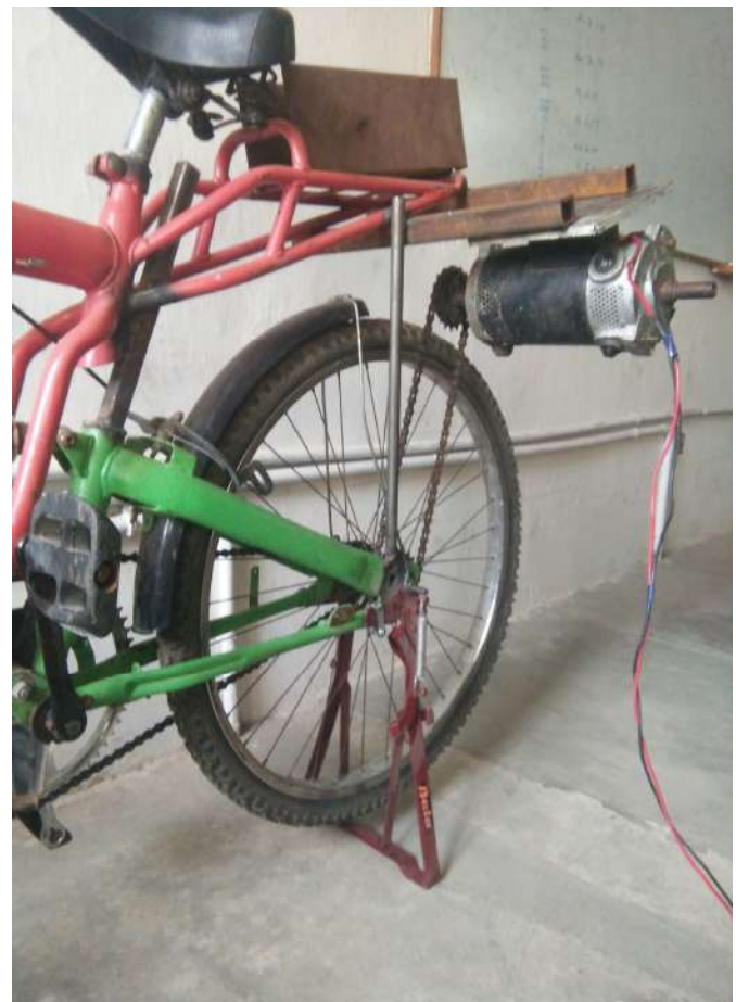
Figure 4. Bicycle coupled with geneartor
