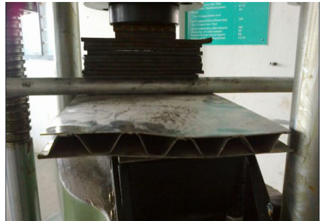
Figure 6. Experimental test of three point bending test
