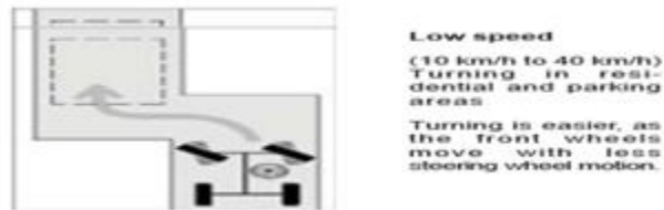
Figure 12. 4-WS drive at low speed [10]
