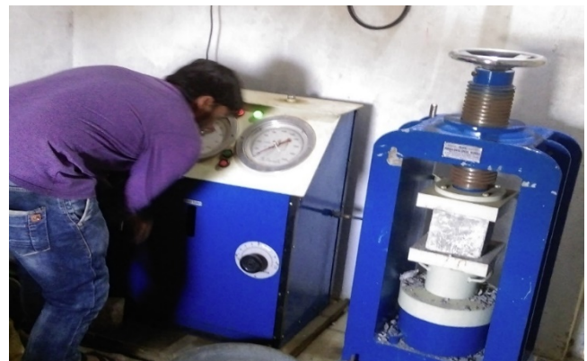
Figure 1: Concrete Cubes Strength Test
