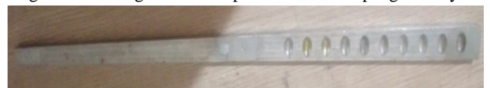
Fig No.14 Divergent plate with Inline arranged Elliptical dimple geometry
