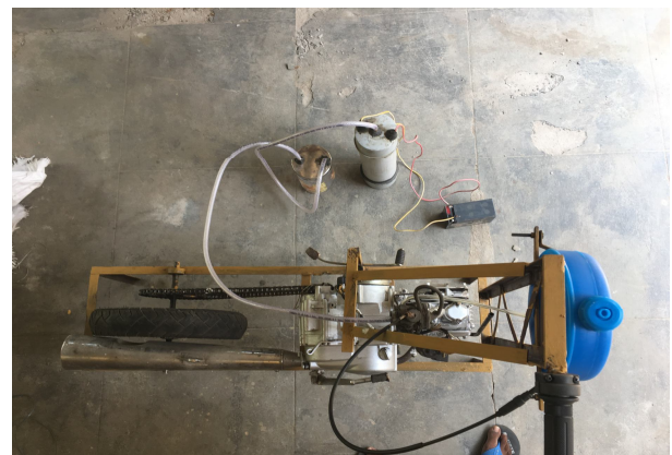
Figure 11. Schematic view of Hydrogen engine (Two wheeler)
