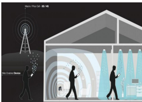
Figure 5. Data transfer by radio waves and visible light
