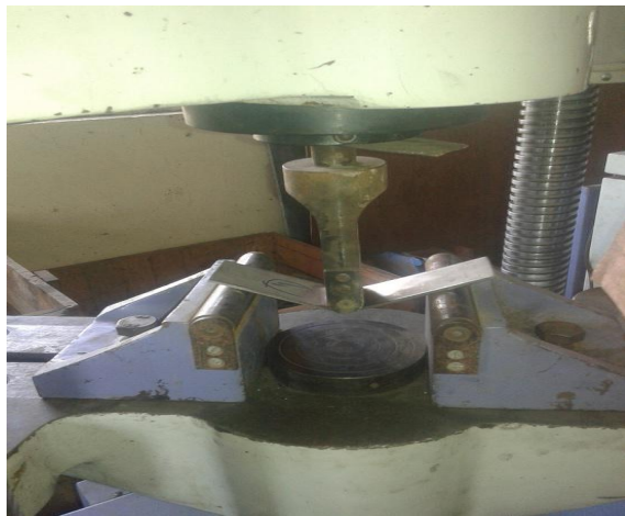
Fig.4Three point bend test
