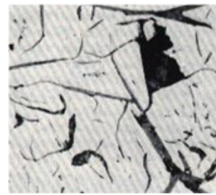
Type C: Superimposed flakes of various sizes, random orientation
