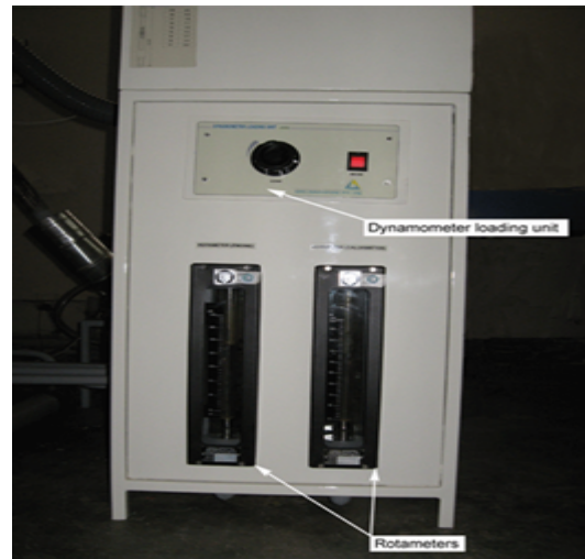
Figure 2 Reading Panel (Fluid Flow, RPM, Load, Manometer, Rotameter & Loading)
