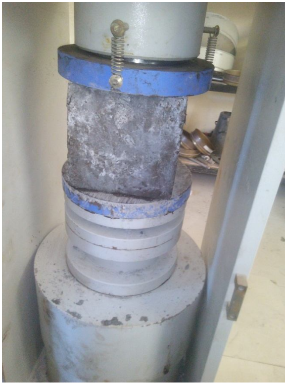
Fig.3 compressive test on specimen.
