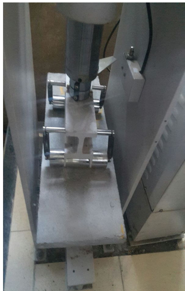
Fig.2 flexural test on specimen
