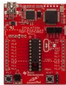
Figure 2. The MSP430 is a mixed-signal microcontroller family from Texas Instruments. Built around a 16-bit CPU, the MSP430 is designed for low cost and, specifically, low power consumption embedded applications.
