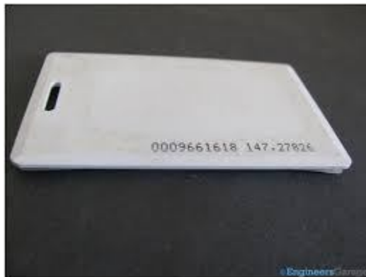
Figure 4. RFID (Radio-frequency identification uses electromagnetic fields to automatically identify and track tags attached to objects. The tags contain electronically stored information. Passive tags collect energy from a nearby RFID reader's interrogating radio waves.
