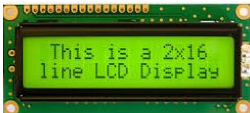
Figure 5. LCD (liquid crystal display) is the technology used for displays in notebook and other smaller computers. Like light-emitting diode (LED) and gas-plasma technologies, LCDs allow displays to be much thinner than cathode ray tube (CRT) technology.
