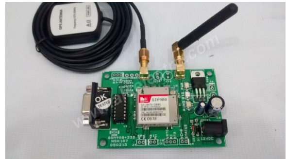
Figure 5 GSM & GPS (Global System for Mobile communications) is an open, digital cellular technology used for transmitting mobile voice and data services. The Global Positioning System is a satellite-based
