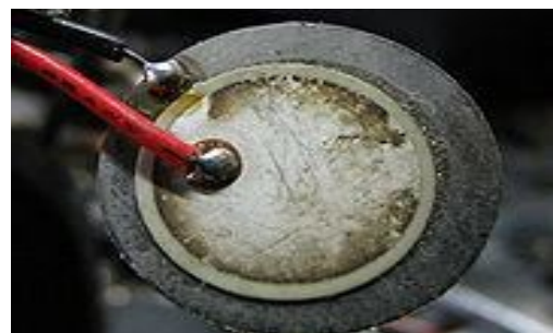
Figure 6. A piezoelectric sensor is a device that uses the piezoelectric effect, to measure change in pressure, acceleration, temperature, strain, or force by converting them to an electrical charge.
