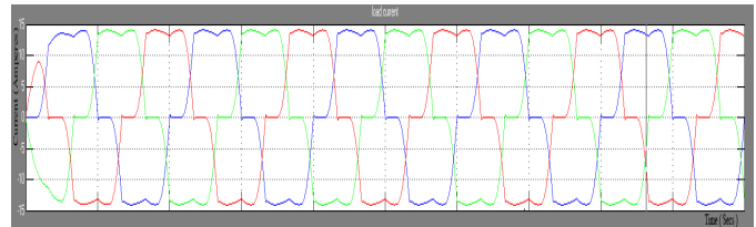
Figure 3. Simulation waveforms after compensation (c) Filter current
