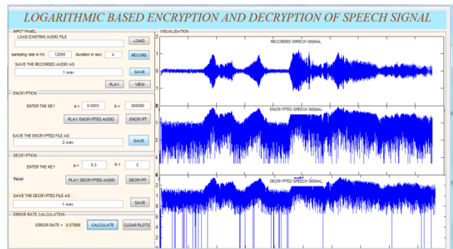
Fig.7 Failed Decryption of ciphered audio sample without the right secret key
