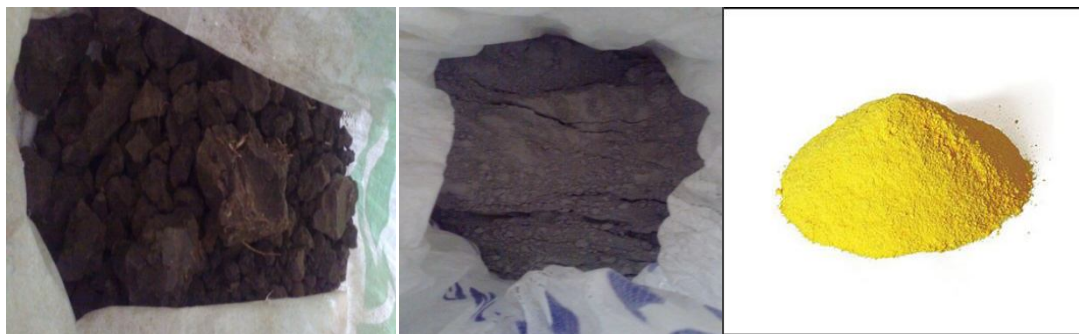
Fig.1 Expansive Soil Fig. 2 Barites Powder Fig.3 Aluminum Chloride
