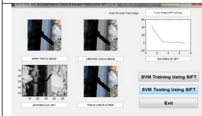
Fig 6.3 Recognition of Large Crack using SIFT and SVM
