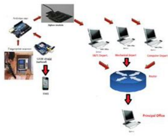
Figure 1 ZigBee based student attendance system
