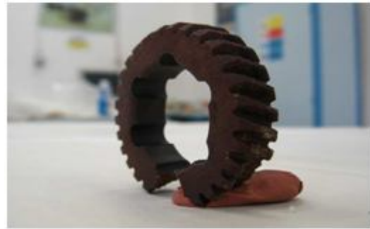
Fig. 9. Damaged Gear wheel
