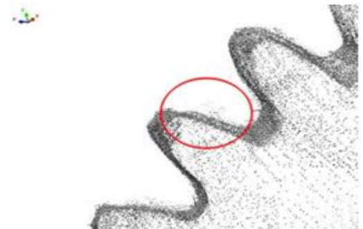
Fig. 10. Inaccuracy of 3D scanning
