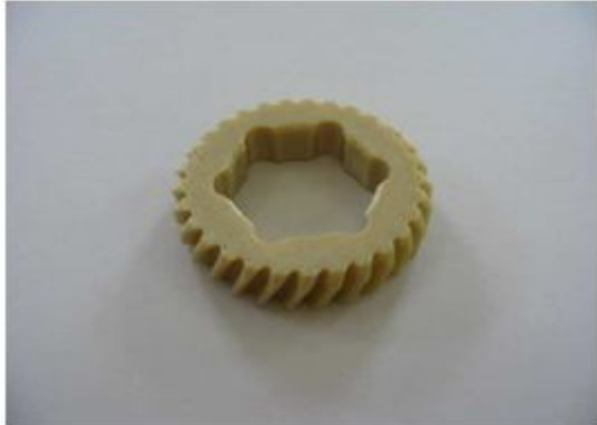
Fig. 14. New gear Wheel made from ULTEM 9085
