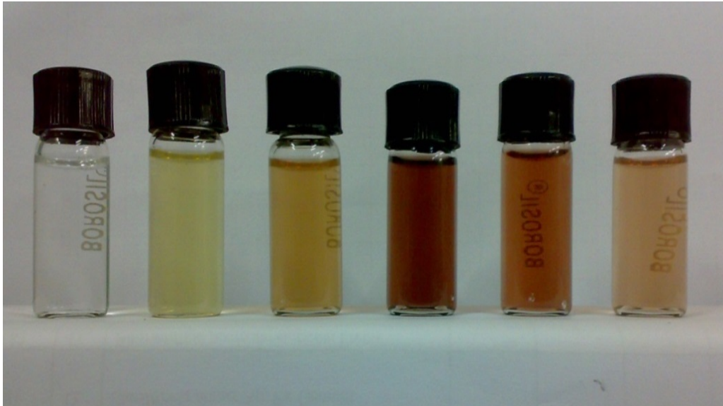
Fig. 3. Silver nitrate ( \text{AgNO}_3 ) solution and colour changes during the reduction of \text{AgNO}_3 into AgNPs by the extract of Gracilariafoliifera after 24 h of incubation
