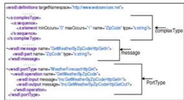
Fig. 3. An excerpt from the Weather Forecast Web service( http://www.webservices.net/WeatherForecast.asmx?wsdl ) that shows the structure of types, messages, and ports.
