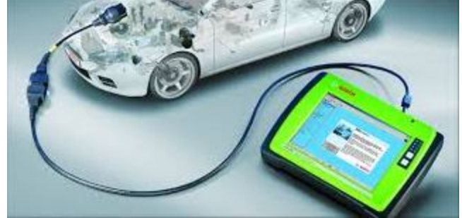
Figure 1: Traditional vehicle diagnostics set up
