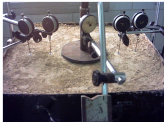
Figure 4. Plate loading test at 25 cm base thickness.
