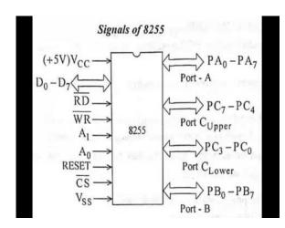
The i8255 provides 24 parallel input/output lines, but the functionality of the i8255 is now mostly embedded in larger VLSI processing chips as a sub-function .The i8255 is still made and is often used to expand micro controller input/output.
