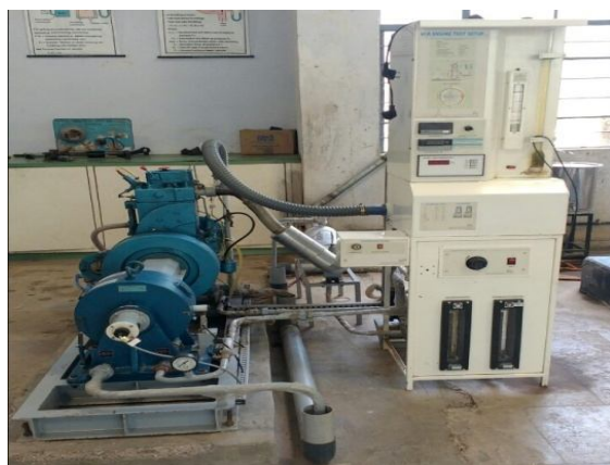
Fig.1.Vcr Engine Test Setup
