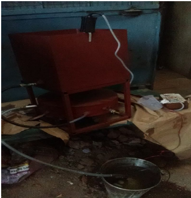
Fig.2.Polymer spiral tube heat exchanger set up.
