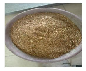
Vermiculite is a light-weight and cheap product that, because of its thermal resistance has become a valuable insulating material. Used as an aggregate with Portland cement it forms an ultra light weight concrete with an open structure ideal for void filling, suitable for use in most light industrial and domestic applications where thermal insulating and fireproof properties are required.
