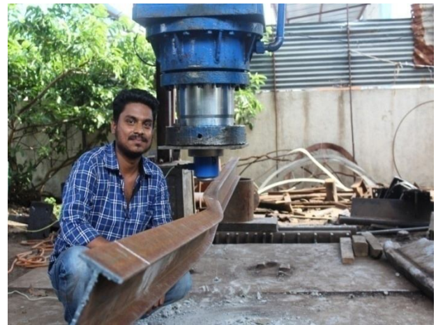
Photo No.3.7 bending of beam after load removes.
