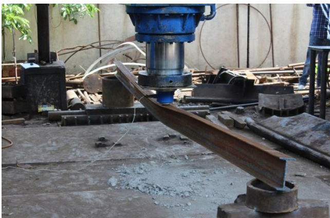
Photo No. 3.6: Beam started bending as load increases.
