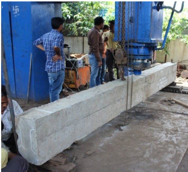
Photo No. 3.1: RCC beam rested on simple support.
