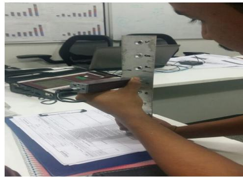
Measurement of Surface Roughness of Aluminium
