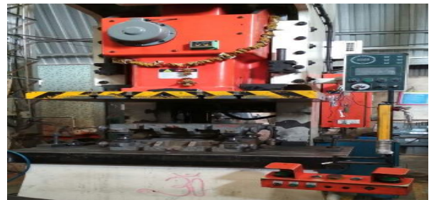
Figure No. 3: Double acting hydraulic press 200 tones.
