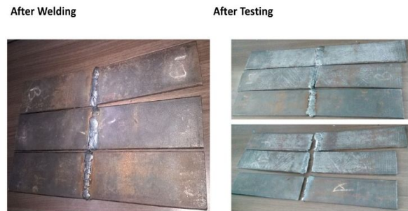
Fig-7 Show the Specimen after welding & after testing
