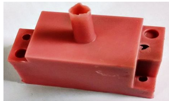
Figure7. Relay produced by wax injector at optimum parameter
