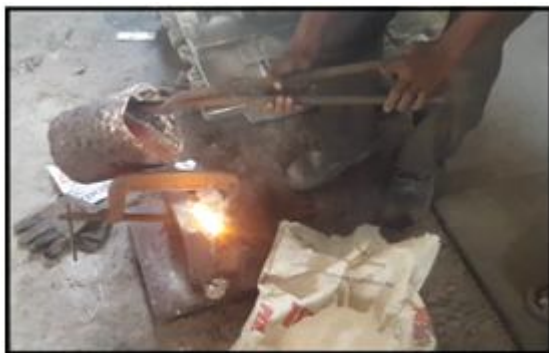
Fig3 Composite mixture pouring into the mold
