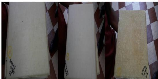
Fig3: Laminates of 0%, 1%, 3%, 5% Clay of NanoComposite
