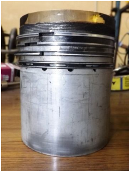
Fig. 2 Photo Graphic View of Aluminium Piston with Brass Crown and Air Insulation
