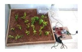
Here the soil is tested using soil moisture sensor, if it is wet then the pump will OFF or if it is dry then automatically the pump will be ON.
