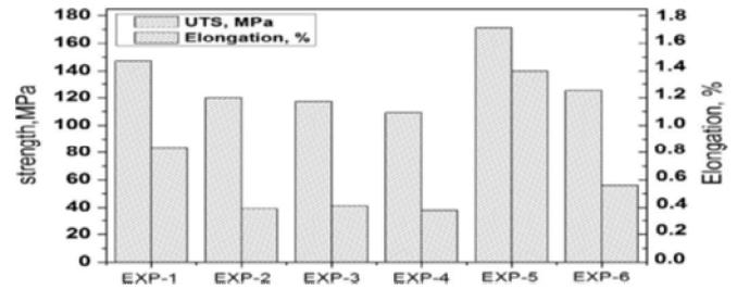
The tensile properties of the composites fabricated under different methods.
