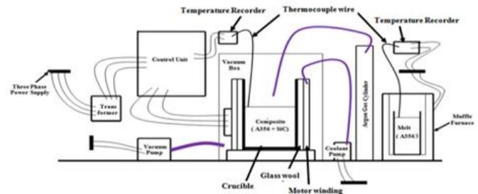
Schematic view of electromagnetic stir casting set-up
