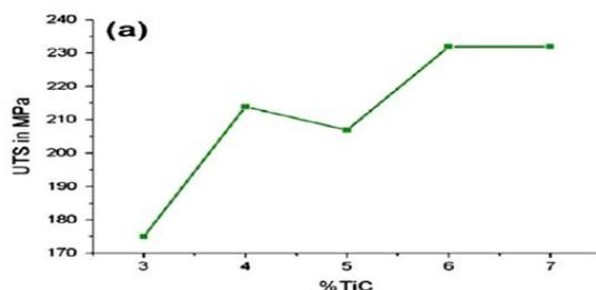
Effect of TiC addition on the mechanical properties of AMC.
