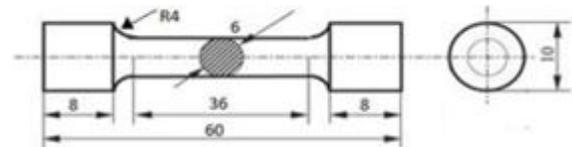
Dimension for the testing of tensile strength specimen
