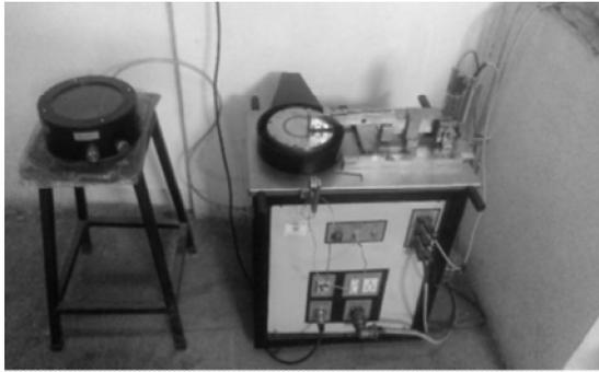
Pin-on-disc type tribo-setup.
