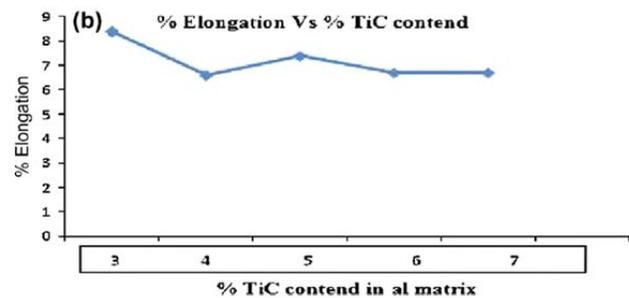
Effect of TiC addition on the mechanical properties of AMC.
