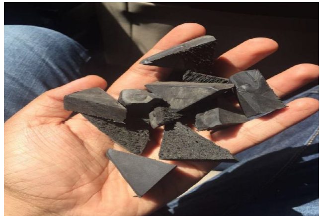
Fig. 3 Angular rubber aggregates of less than 12 mm
