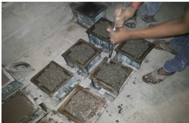
Fig. 5 Tamping the concrete while casting the cubes
