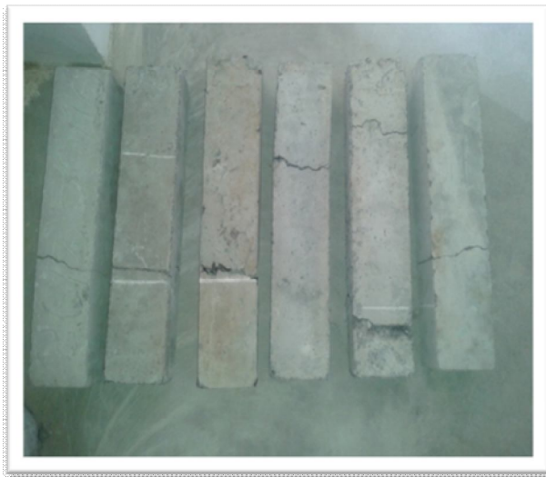
Fig. 6 Flexural Strength test on Concrete
