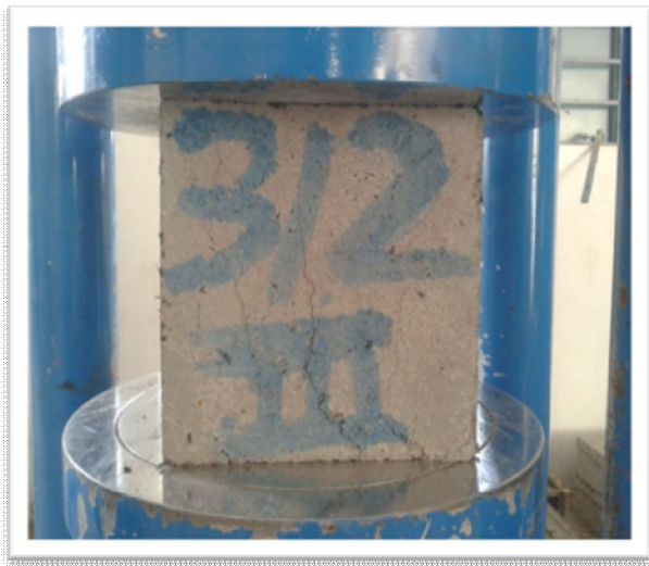
Fig. 2 Compressive Strength test on Concrete
