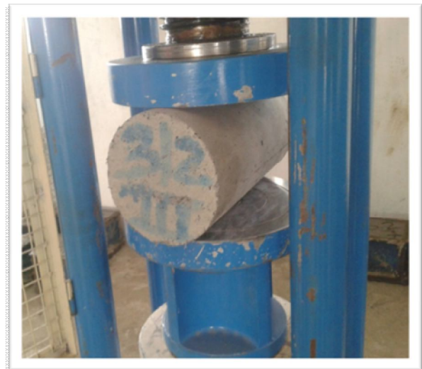
Fig. 4 Split Tensile Strength test on Concrete.
